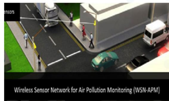
These low-cost sensors will be highly useful to monitor the air pollutants, map the air quality and can be used as Early Hazard Warning System for air pollution episodes in a city. Measurement of vehicular & industrial pollution and hazard identification at hazardous sites is much more convenient with the help of sensor-based real-time monitoring networks. These sensor-based monitoring networks shall be the in-thing for India's air monitoring program.
